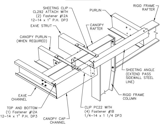
NOTES: ALL BOLTS TO BE  $\frac{1}{2}$  "Ø UNLESS NOTED. FOR REQUIRED LENGTH REFER TO GRIP TABLE ON CUSTOM ERECTION DRAWINGS.
